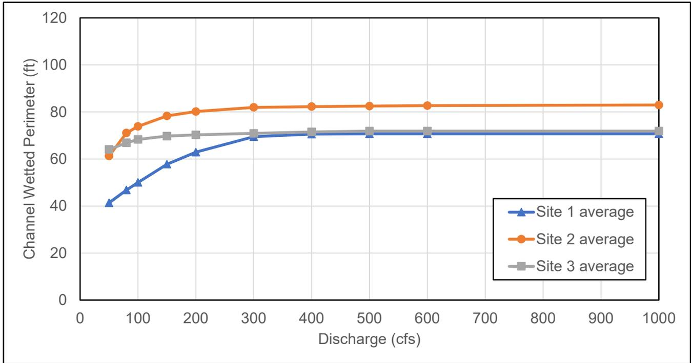
Figure 43. Run habitat type rating curve for channel wetted perimeter
