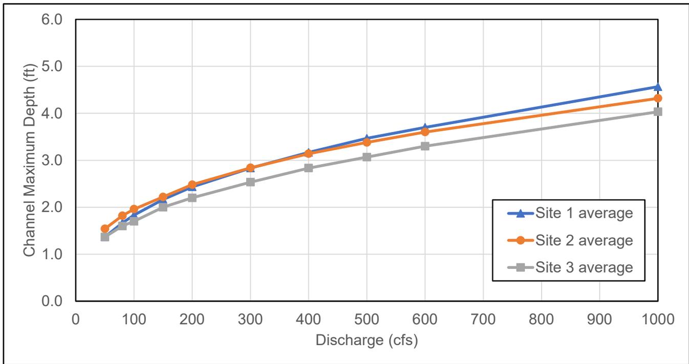
Figure 45. Run habitat type rating curve for channel maximum depth
