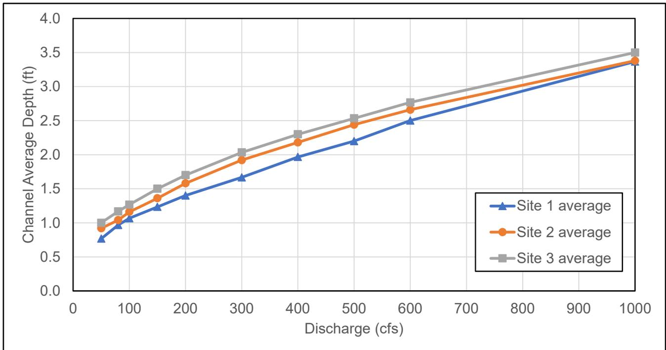
Figure 44. Run habitat type rating curve for channel average (hydraulic) depth
