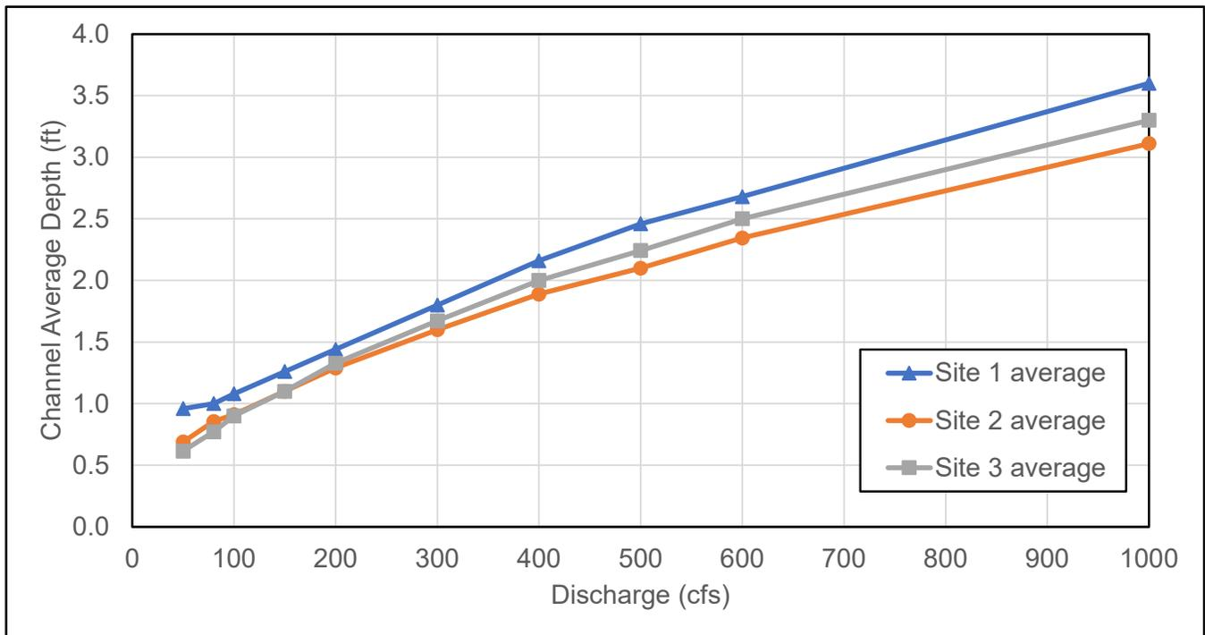
Figure 41. Riffle habitat type rating curve for channel average (hydraulic) depth
